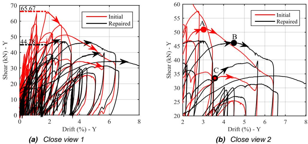
**Figure 6:** Comparison of the hysteretic response of the initial and repaired column in Y axis
