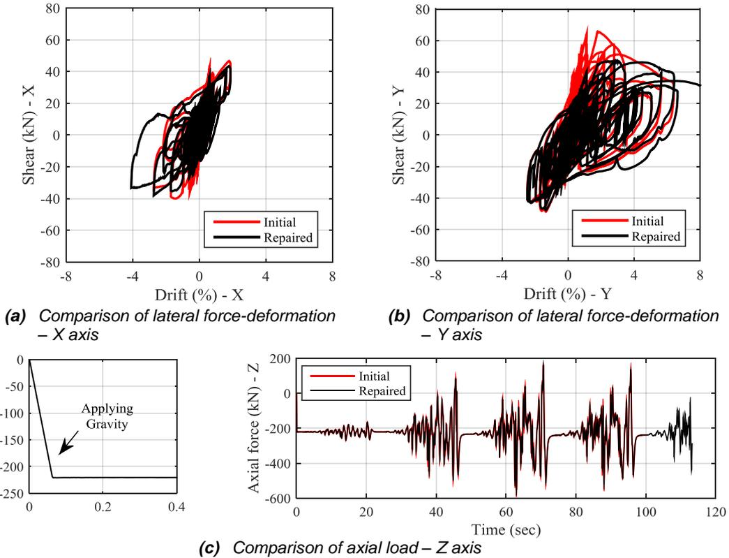
**Figure 5:** Comparison of hybrid simulation test results between initial and repaired RC column
