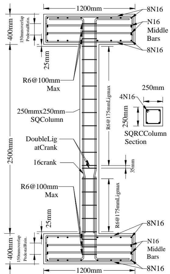
Figure 4: Design details of the specimen
