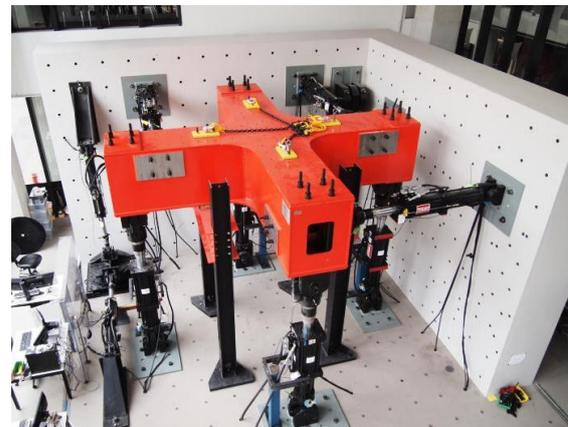
**Figure 2: Multi-Axis Substructure Testing (MAST) system in Smart Structures Laboratory at Swinburne University of Technology**
