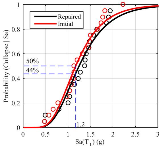
**Figure 7:** Comparison of fragility curves for the initial and repaired RC columns
