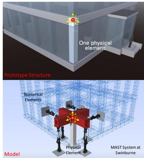
**Figure 1: Hybrid simulation technique**
